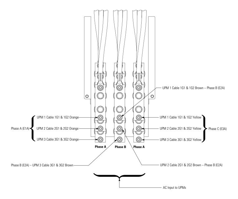
NOTE Two cable lugs will be connected to each terminal stud. When connecting the cable lugs, install the first lug on the stud with the raised barrel portion facing the back of the cabinet. Install the second lug with the raised barrel portion facing the front of the cabinet.
